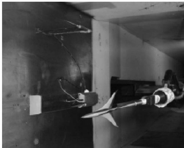
Figure 6. View of the model mounted in the wind tunnel.
